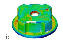
**Tested for accuracy**We have verified dimensional accuracy within ±0.2 mm or ±0.2% nominal length
