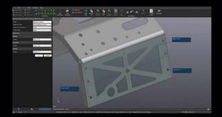
Before starting the dimensional inspection process, the position and orientation of the object in space is of utmost importance. It ensures more accurate results from data acquisition up to the final inspection report.
