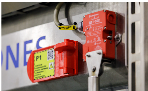
3D printed safety lock preventing machines from starting up during maintenance
