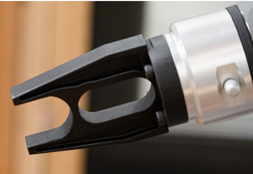
The company has printed end effectors for their robots to conduct numerous tests
