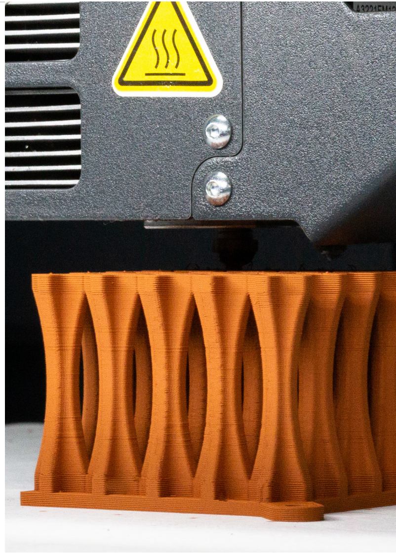
Heatsink 3D printed in pure Copper.
