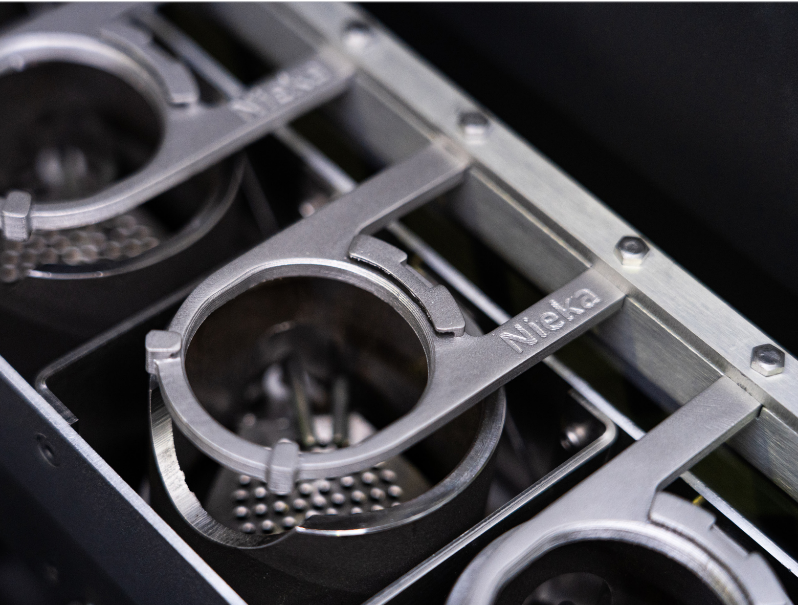
3D printed Inconel 625 crucible clips from Nieka Systems.
